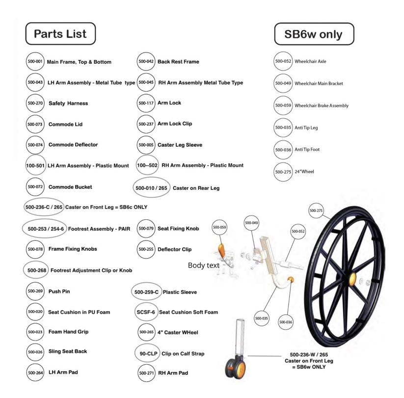
This Universal Parts List for SB6c and SB6w includes original and updated design components. Check the exploded parts diagram to obtain the correct part for your chair. if unsure contact your supplier.
